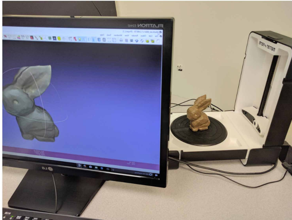
Figure 3. The matter and form 3D scanner used in this project
