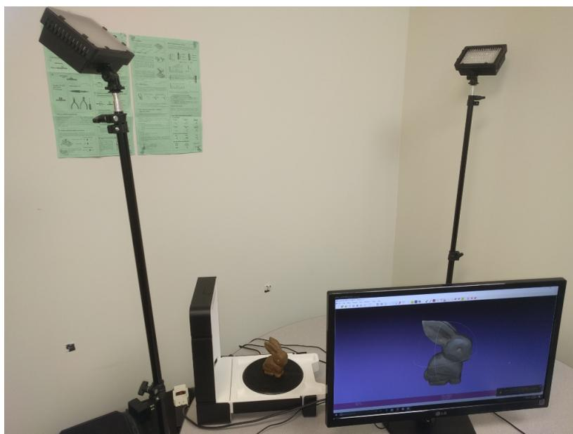
Figure 1. 3D scanner and lighting set up.
